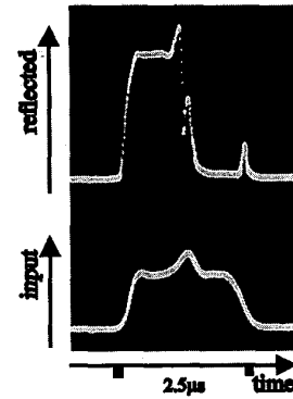
CFC6 Fig. 1 Input and output pulses showing the bistable memory effect, with a switching contrast of 30:1. The input plateau is 0.9 mW.
